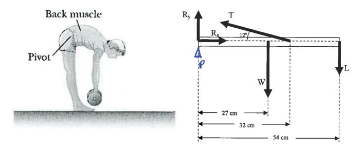
The spine and upper body are represented as a uniform horizontal rod of 41.5 kg (W) pivoted at the base of the spine. The erector spinalis muscle acts at an angle of 12° to maintain the position of the back.
