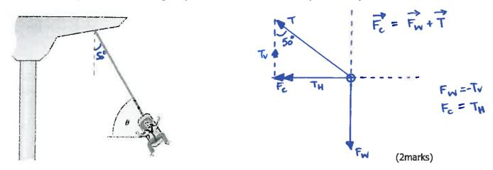
Once the carousel is turning at full speed the chain typically makes an angle of 50° with the vertical. You can assume that for this example the combined mass of the chair and passenger is 115 kg and that the radius of revolution is 15.2 m.
